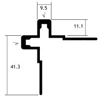
Part #110184 38.1mm Radius Cover Trim This trim allows you to soften a harsh corner while providing a durable and protective edge.
